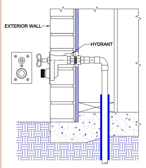
The Wade 8601 wall hydrant provides an anti-siphon installation in any type of wall construction. The water supply piping is first run to an elevation above the finished floor level at the anticipated hydrant location. The piping should be insulated for protection against aggressive soils and concrete. The type of piping and connections are irrelavent - a standard 3/4" NPT threaded adapter is all that is required. The piping should be accessable for connection after the concrete is poured.
