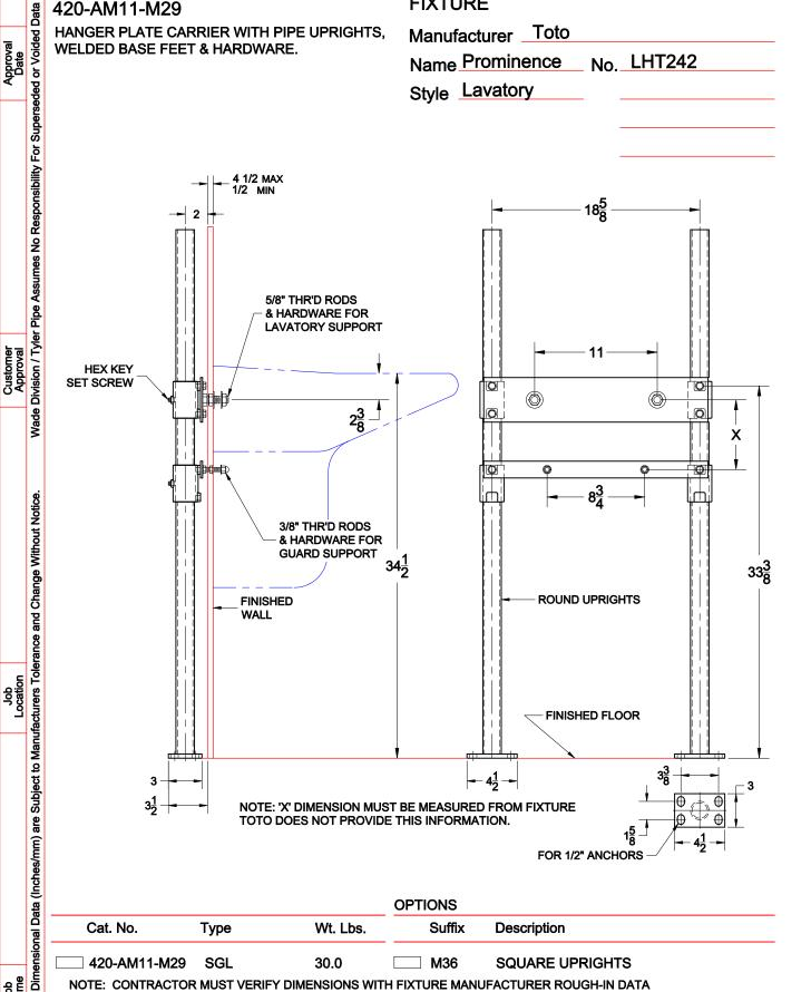
**OPTIONS** Cat. No. Type Wt. Lbs. **Suffix** Description SGL 3 420-AM11-M29 30.0 **SQUARE UPRIGHTS** NOTE: CONTRACTOR MUST VERIFY DIMENSIONS WITH FIXTURE MANUFACTURER ROUGH-IN DATA TYLER PIPE / WADE DIVISION ACCEPTS NO RESPONSIBILITY FOR ANY INACCURACIES IN DRAWING
